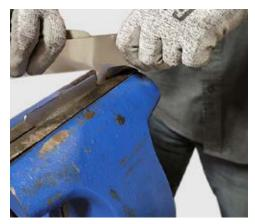
3. Using both hands rotate the top of the plate 90 degrees
