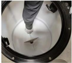
5. Place finished anti-vortex plate inside the tank
