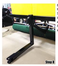
8. INSTALL HITCH: Install (1) 5/16" Nut on each of the two remaining 5/16" Bolts and loosely screw them into the nuts on the Mounting Frame as shown in the image to the left. Adjust height as needed for your application.
