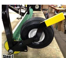
7. INSTALL LIFT ARMS & TIRES: Install Lift Arms as shown in **Image above** using one 1/2" Washer and one 1/2" Lock Nut. (Note: Overtightening nuts will make arms difficult to move.) Next, slide Axle Bushings on axles as shown in **Image 7a**. Finally, install tires as shown in **Image 7b** using one 5/8" Lock Nut.
