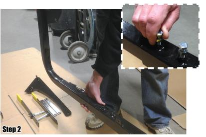
2. INSTALL ROLLER ARMS: Slide Roller Arms into both ends of the receiving tube on frame as shown in **Image 2**. Install one 5/16" Nut on each of four 5/16" x 1" Bolts and loosely install them into the welded nuts on the frame as shown in **Image 3**. (Do not tighten yet.)
