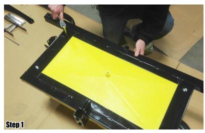
1. <u>INSTALL FRAME ON TANK:</u> (Make sure the "decal side" of the tank is opposite the hitch side of the frame - See Cover Page.) This step uses the (4) 5/16" x 1/2" Flange Bolts.
